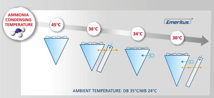
15K REDUCTION at equal capacity and equal sound level
