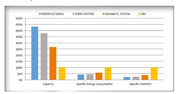
The capacity increase starting from the dry system is very significant. Specific power draw is greatly reduced ensuring energy saving up to 60% compared with a dry unit. Important reduction of footprint (up to -80%).
